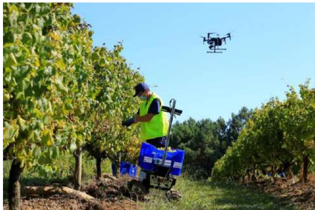
Figure 16: CSIC, CAR presented a grape robot: Robert (acronym for 'Robot for collaborative manual harvesting') that allows human workers to focus on the task of collecting the fruit while the robot provides the physical strength.
