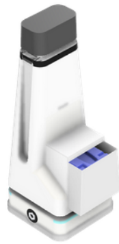
Above: Harmony robot prototype - two modules version (3D drawing). As it is a modular robot, it can be added another storage space on the back, for the transportation of bigger objects.
