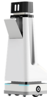
Above: Harmony robot prototype - Simple version (3D drawing). In this image, the robot is in its simplest form, with only front storage, for the delivery of small objects.
